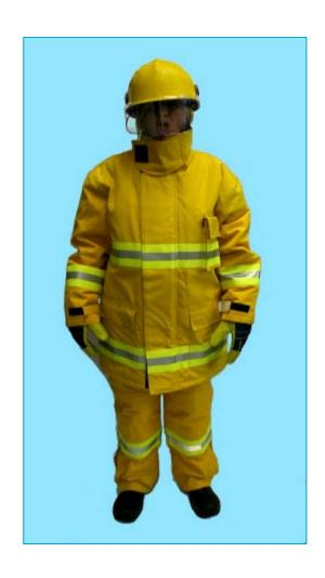
The Fire Cheater High Performance Suit is made up of a multi-layer structure of NOMEX as the outer shell, lined with CONEX and TWARON moisture barrier, insulating thermal barrier layer and flame resistant lining.
