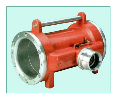
Designed for connection to water delivery hose. For the cleaning of mud, gravel, sand and dirt. Soiled hose is pulled through the attachment, whilst the water connection to the washer feeds two internal pressure jets, which clean the outer jacket of hose. The impact of the water from the jets propels the hose forwards. Suitable for hoses with diameter up to 76mm.
