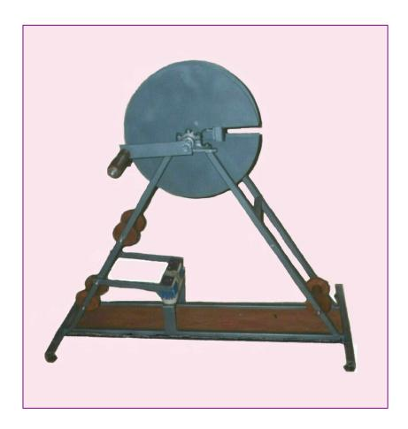
Proper care of fire hose after use pays for itself in a very short time through increased hose life. Our hose winding and brushing machine, used extensively by fire brigades all over the world, performs the job neatly and efficiently.
