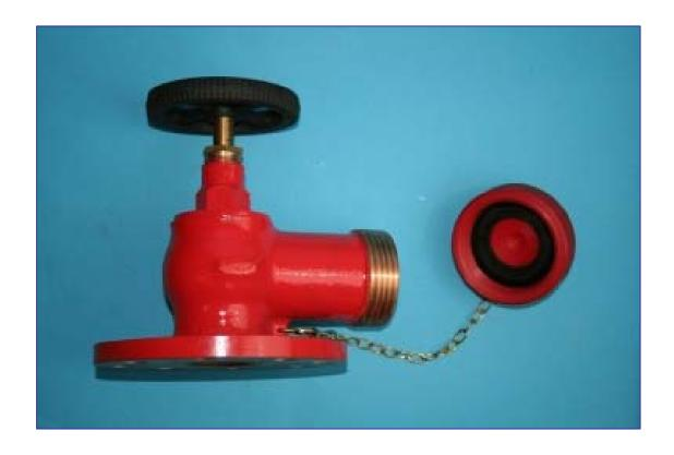
The Valves are manufactured in corrosion resistant materials with an LG2 gunmetal body, cast iron handwheel and plastic plug and chain.
