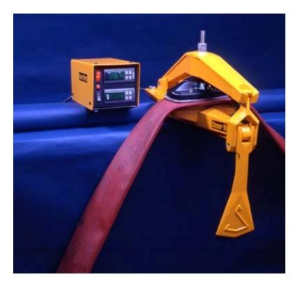
A Vulcaniser developed for the repair of fire hose, with an adjustable temperature set-point, allowing the vulcanisation/welding of all fire hose materials. Electronic temperature control, to within 1°C of set point, and electronic timing give the operator total control over pre-heat, curing temperature and time. This ensures high quality, repeatable repairs and eliminates hose scorch.
